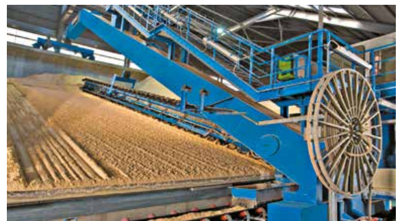
Semi-Portal Scraper Reclaimer
